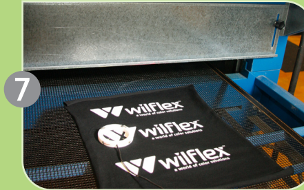
7 Validate the cure temperature by running a test print through the dryer using the same belt speed as the production run.
