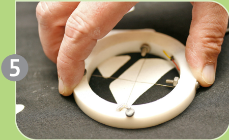
5 Position the probe over the area with the most ink density.
