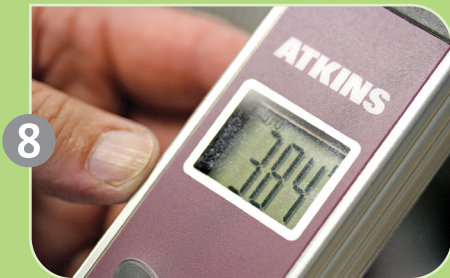
8 Carefully monitor the display as the print moves down the dryer tunnel. Make sure the peak temperature meets or exceeds the recommended cure temperature for the ink(s) being used.
