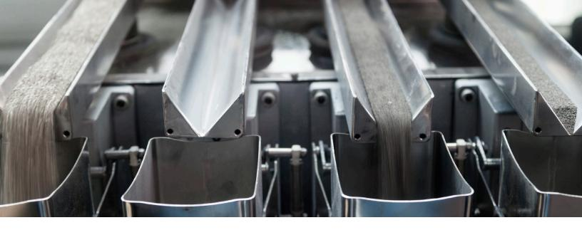
Avient's composite springs are manufactured using a continuous pultrusion process. Resin impregnated, continuous glass fibers are drawn through a curing die of a specific cross section, yielding consistent quality, dimensions and mechanical properties to provide more consistent spring rates than alternate materials. Reinforcement fiber configurations are designed to provide high flexural strength and modulus in the axial direction plus fastener bearing strength in the transverse direction.
